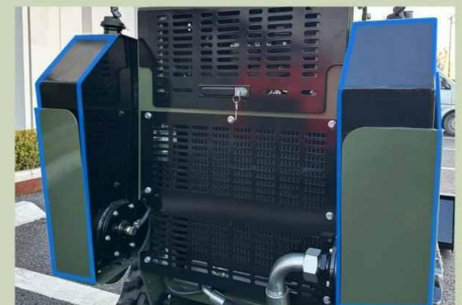
**There are protective fences** on both sides of the driving weighing to prevent the operator from being injured by splashed materials or debris during the operation.
